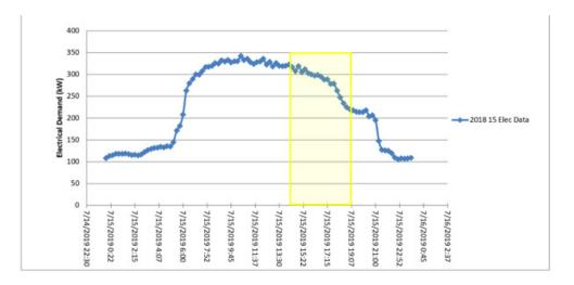
Figure 9. GSA office building electrical load profile
